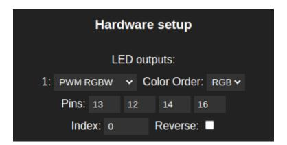
Change the output pins to match your LED strip, often the Red and Green change depending on LED strip manufacturer. Setting the relay output to pin: 4 controls the LED on the PCB and Wemos D1, turning it on and off as the WLED mode is turned on/off.
